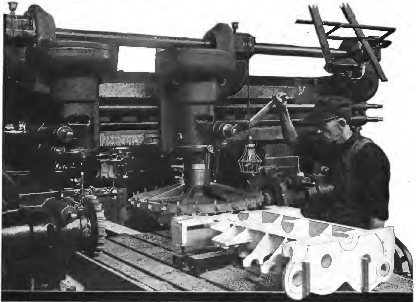
Ingersoll crankcase milling machine used by the Haynes Automobile Company, Kokomo, Ind.
